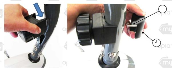
12. Bring the vertical handlebar (19) into position against the front mounting tube so the handlebars are facing up and towards the rear of the machine, and the brackets are aligned. Then, attach it using the 2 pre-assembled screws (20) and lock washers (21) and tighten (rotate right) using the Allen key, then clip the cover (22) into position.
